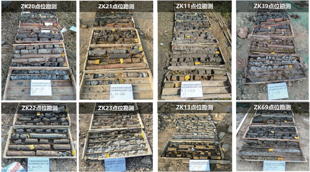
图 3 地勘钻孔岩芯与土壤取样 Fig.3 Geological drilling core and soil sampling
